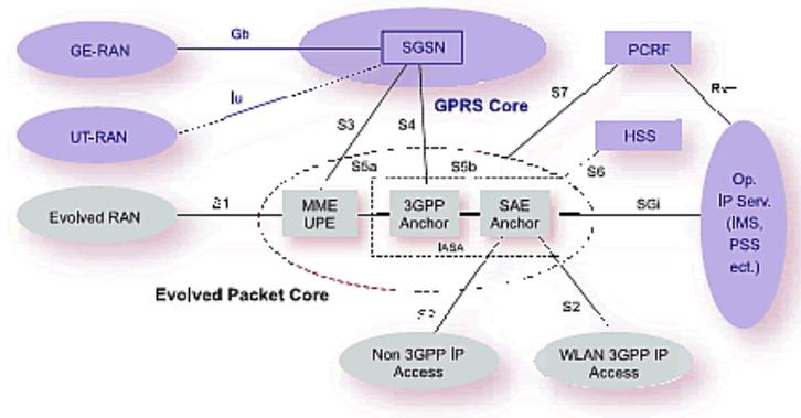
LTE targets requirements of next generation networks including downlink peak rates of at least 100Mbit/s, uplink rates of 50 Mbit/s and RAN (Radio Access Network) round-trip times of less than 10ms. LTE supports flexible carrier bandwidths, from 1.4MHz up to 20MHz as well as both FDD (Frequency Division Duplex) and TDD (Time Division Duplex).
